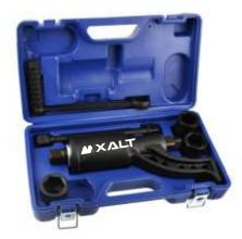
A torque multiplier uses a planetary gear system, or epicyclic gear train. As you turn the input shaft, the output shaft slightly rotates. It takes 65 turns of the input shaft to turn the output shaft just once! With a 1:65 output ratio. This small, light tool is an ideal addition to the basic tools provided for every industrial vehicle, agricultural vehicle, bus, etc.
